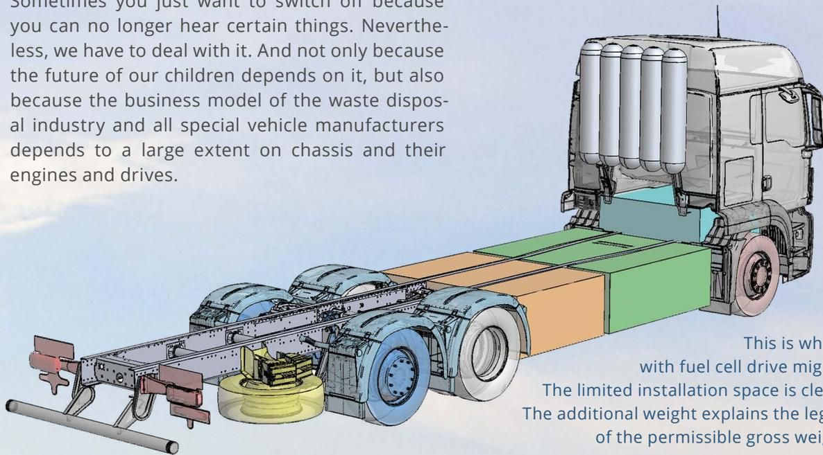
This is what a chassis with fuel cell drive might look like. The limited installation space is clearly visible. The additional weight explains the legal increase of the permissible gross weight by 10%.
